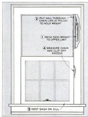
8 Chain can be cut to correct length by pulling weight to top of its travel, fastening, and measuring with sash resting on sill.
